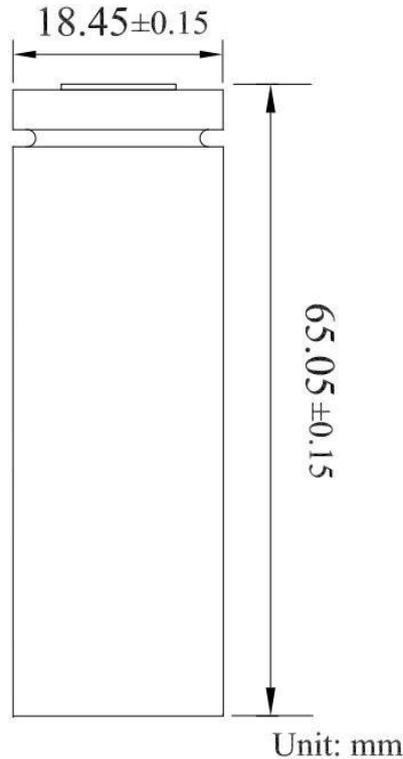
Fig.1 Outline Dimensions of KHINR18650-3200mAh 3C(with tube)
